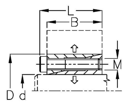
B mm = 17d mm = 16.00D mm = 32Fit tolerance = Aksel h8, Nav H8 F kN torque = 8.0L mm = 21.0M mm = M4P N/mm2 surface pressure on shaft/hub = 65 Surface roughness = R? ?  $3.2 \mu m$ T N m torque = 70Ts N m bolt tightening torque = 4.9
